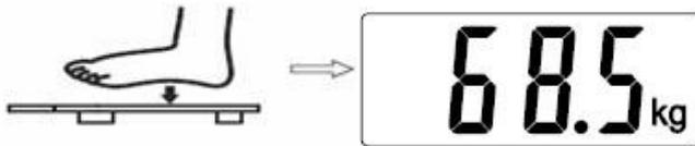
2. The factory default unit is “kg” , if not applicable, please set switch on the back of scale to choose the needed unit lb or st.
